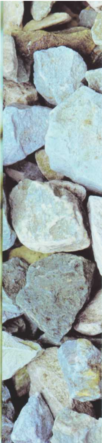
• The pre-filtration material is often coarse, in order to trap the bulkiest particles.
