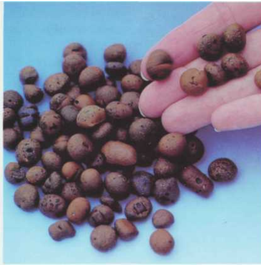
Balls of clay can be used for pre-filtration.
