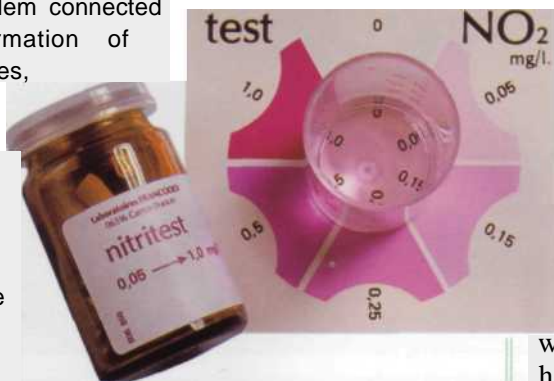
The darker the pink color, the more nitrites there are in the tested sample.
