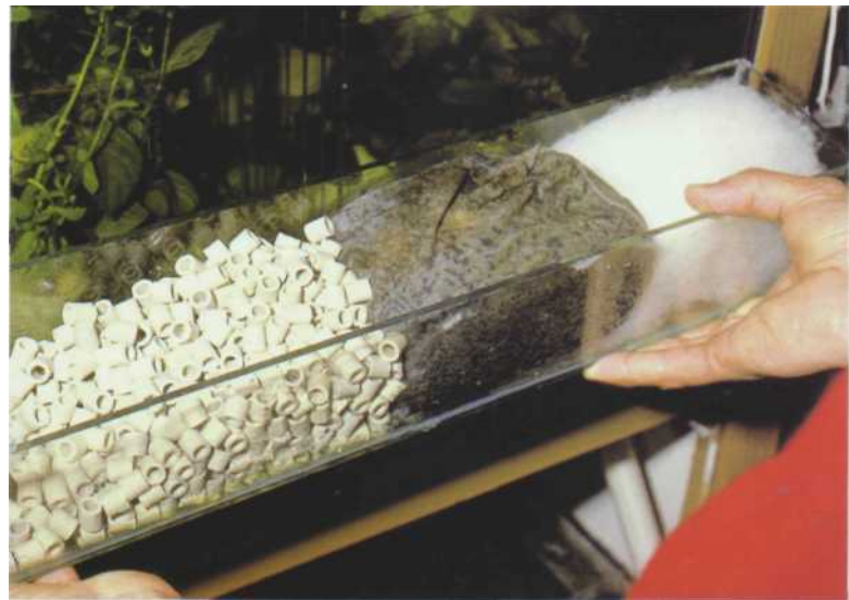
Gutter filter equipped with thick filtering media (left) and finer ones (right). V
